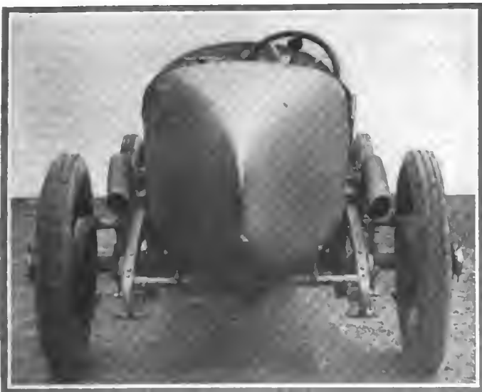
Tapered tail of special Packard chassis. Note the two exhaust manifolds
